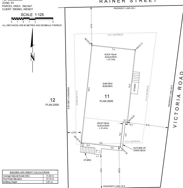
ELEVATIONS ARE GEODETIC AND DERIVED FROM CONTROL MONUMENT 77H5231
